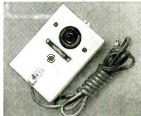
A new "adjustable" Line-Filter or balancer which is connected between the A.C. line and the receiver itself. (No. 513)
